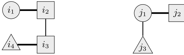
Fig. 2 An example of the first two rounds of an IKEP with N = \{1, 2, 3\} . Round 1 is displayed on the left, and round 2 on the right. In this example, both rounds are the same, irrespectively of the solution concept that we use for the initial allocations. This is because round 1 has a unique maximum matching
