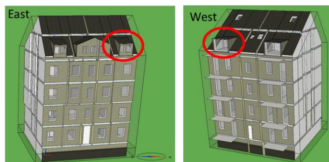
Figure 4: 3D model of the selected GZH building in the thermal building simulation tool IDA ICE. The analysed bedroom (east façade) and kitchen living room (west façade) are labelled with red circles
