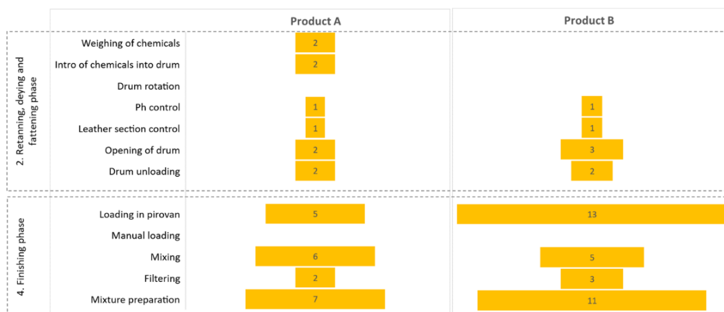
Figure 6. N. of activities with non-negligible risk index ( 15 \leq R < 21 ) in LC processes & phases of A and B products.
