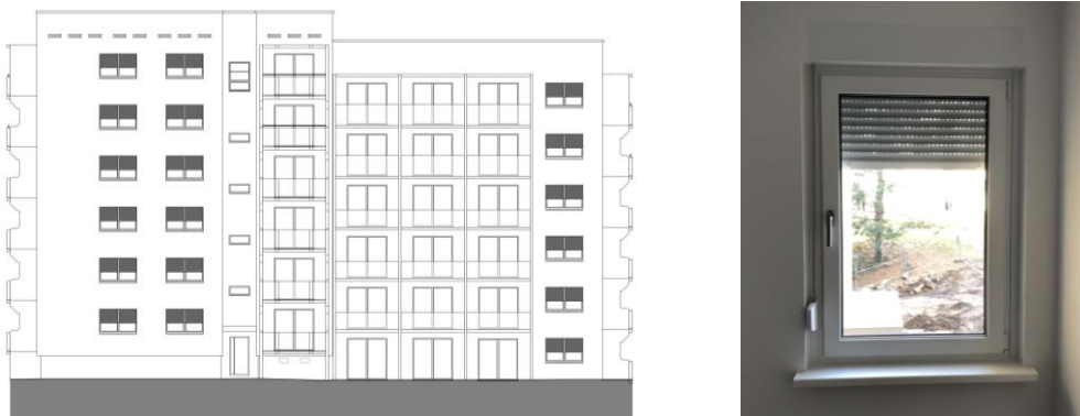
Figure 8. External shading devices on the windows, left: southern façades with planned adaptation measures. Reference: IGC Ingenieurgesellschaft Cossebaude GmbH (2018), right: window after implementation of the roller shutters.
