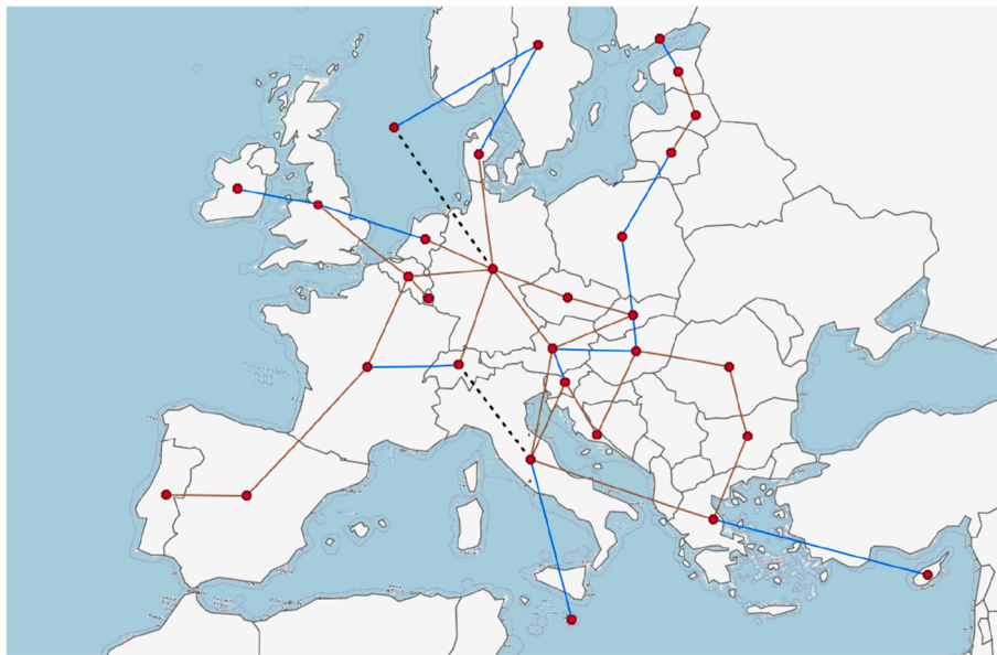
Fig. 6. Hydrogen transmission infrastructure by 2050, E-Fuel_80 scenario (blue lines: dedicated hydrogen; brown lines repurposed gas pipelines; dashed lines: blending). (For interpretation of the references to colour in this figure legend, the reader is referred to the Web version of this article.)
